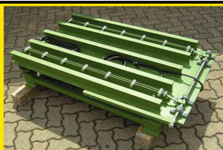
Vibrating table with integrated transport mechanism
